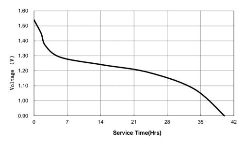
Discharge method:1k $\Omega$ , 24hours/day, E.V. 0.9V Temperature: 20±2 $^{\circ}$ C
