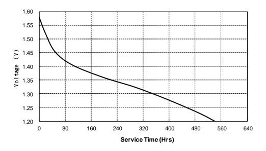
Discharge method: 15k $\Omega$ , 24hours/day, E.V. 0.9V Temperature: 20±2  $^{\circ}$
