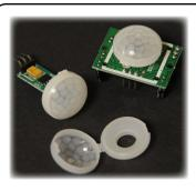
Low voltage sensor modules are available. Sensor modules have analogue pyro with switching circuit and sensitivity sdjustment. Can be combined with relay module for mains switching. Modules can be used for alarm activation or lighting.
