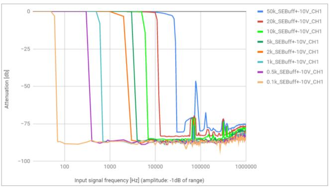
Analog input frequency response - single channel mode, buffered single-ended input, different sample rates
