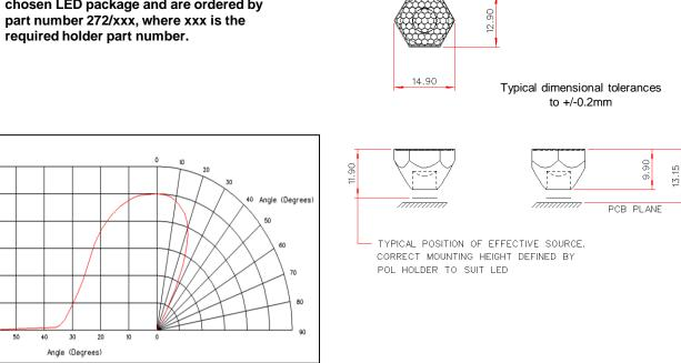
Typical Cartesian/Polar Output Intensity Plot with 1mm die size high Power LED
