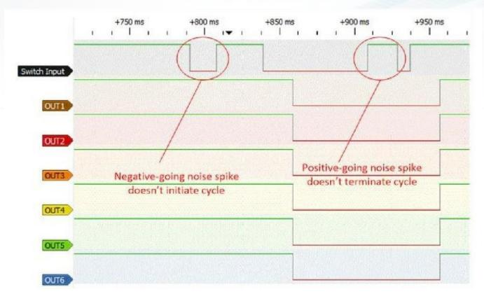
This logic analyzer capture of a LS10 Series IC cycle showing a noisy switch input commonly applied to all six device channels. Note the initial 19 ms High-going glitch at approximately +780 ms does *not* start a cycle, and the folHighing 18 ms high-going first glitch at about approximately +915 ms does *not* terminate the cycle. LS10 Series devices are designed to function flawlessly in severe electrical environments. These devices reject any uninvited level transition of <20 ms duration.
