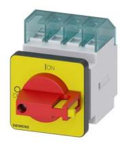
SENTRON, Switch disconnector 3LD, emergency switching-off switch, 4-pole, Iu: 16 A, operating power / at AC-23 A 400 V: 7.5 kW, front-mounted, knob-operated mechanism, red/yellow, 4-hole mounting of the handle
