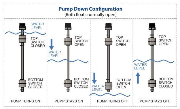
\*NOTE: PUMP DOWN = TURN PUMP OFF WHEN NEAR EMPTY AND TURN PUMP ON WHEN NEAR FULL.
