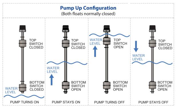
\*NOTE: PUMP UP = TURN PUMP ON WHEN NEAR EMPTY AND TURN PUMP OFF WHEN NEAR FULL.
