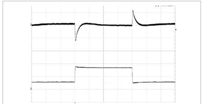
Output voltage response to load current step- change (1.125-3.375-1.125 A) at: T_{P1} = +25^{\circ}\text{C} , V_i = 24\text{ V} , di/dt = 1\text{ A}/\mu\text{s} C_o = 22\text{ }\mu\text{F} ceramic capacitor Top trace: output voltage (200 mV/div.). Bottom trace: load current (2 A/div.). Time scale: (0.5 ms/div.).
