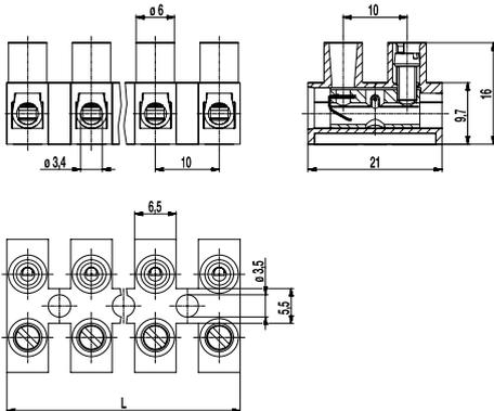
The plug-in terminal strip 323-FB is available in 10 mm pitch with 2 to 12 poles. It has one screw connection per pole and one plug connection for a terminal strip with pins.
