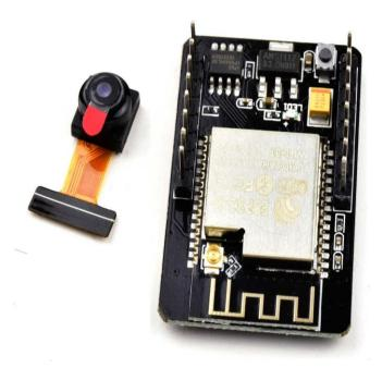
Ai-Thinker ESP32-CAM is a small and ultralow power device with the original Ai-Thinker ESP32-S SoC and an OmniVision OV2640 Camera module with 1600 x 1200 pixel. The ESP32-S SoC contains two 240MHz Xtensa® 32-bit LX6 microprocessor cores, 32Mbit flash memory, and radios for Bluetooth 4.2 and WiFi 2.4GHz.
