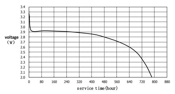
Discharge method:30K $\Omega$ , 24 hours/day EV 2.0V temperature of 20±2°C
